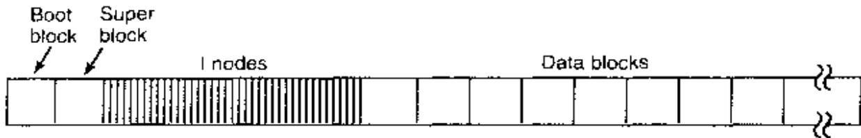
Figure 10-31. Disk layout in classical UNIX systems.
